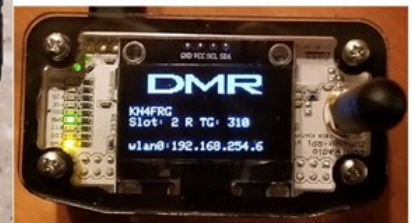
Figure shown with Retevis RT-84 & HRO ZUMspot kit. Note: The ZUMspot can connect To gateways for DMR, D-STAR, etc.
